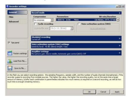
**General Tab** - the tab selects record mode, timers, VAS and in case of Tiny 16+ amplifier's parameters.
