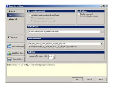
On Recorder Connect (Check box "Download records to default folder") - With the check box selected when connecting the recorder to the PC, the records are automatically uploaded to default folder specified in the field Default Folder.
